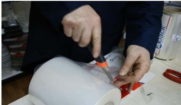
Inner surface of film should face to the mold
